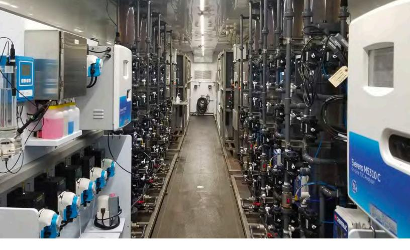
BWW'S MOBILE PILOT PLANT TESTS WATER PROCESS TREATMENT ALTERNATIVES.
