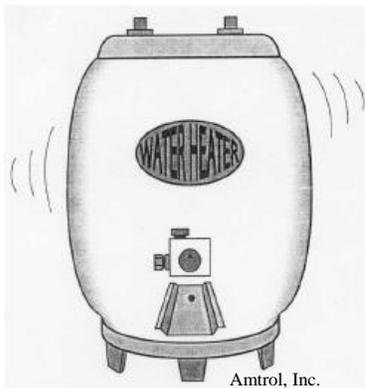
heater tank and household plumbing. Thermal expansion may cause the T & P relief valve to leak, household plumbing fixtures to drip, solenoid valves on the icemaker and dishwasher to malfunction, toilet ball-cocks to leak, or washing machine hoses to burst. Extreme Thermal Expansion may cause serious harm to the water heater, particularly if
